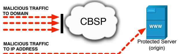
Figure 2: In the case of DNS rerouting, only traffic that uses the domain name is diverted through the CBSP’s network. Traffic that uses the IP address of the protected server can reach the web server directly.
